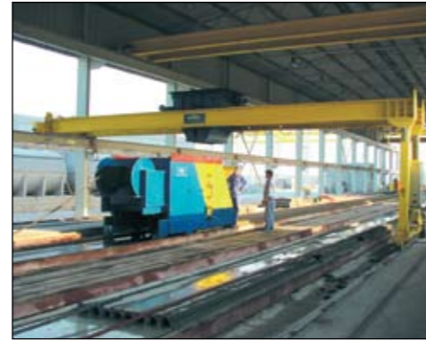
Full Automated Concrete Distributor
