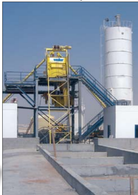
Automated Concrete Batching Plant
